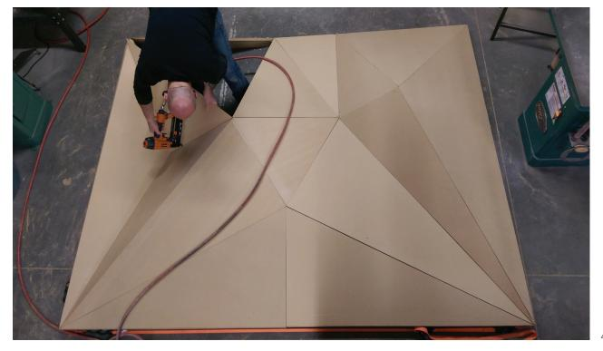
The final façade was broken down into seven triangulated parts that come together to make the final façade assembly. The team re-designed the assembly sets to be CNC milled with 2-dimnesional panels, using the router to digitally control the milled angles in order to join the flat pieces in to triangulated assemblies. This process allowed the panels to come together quickly, reducing weight and shipping costs. The seven forms were sent to Warner
